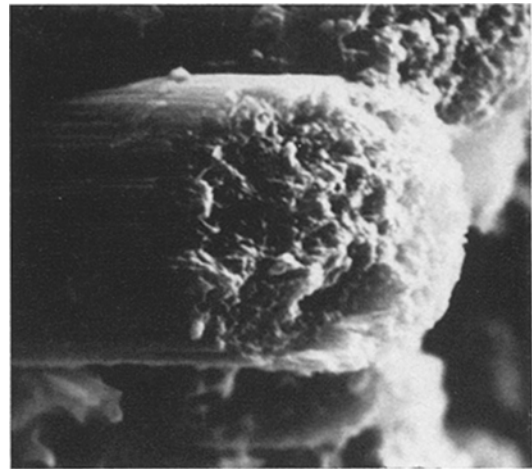
Figure 20 Modulite 5206/Nomex hybrid, lay-up B, transverse impact, unnotched: 90^\circ graphite/epoxy ply, \times 6000 .
