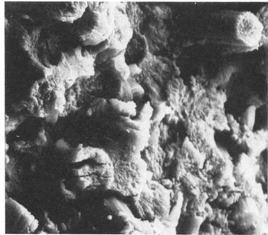
Figure 8 Modulite 5206/glass hybrid, lay-up B, longitudinal impact, unnotched: 0^\circ graphite/epoxy ply near tension surface, \times 1750 .
